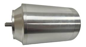
4 poles, Inverter duty Δ/Y 230/400V/50Hz I.CI.F - IP69K - IC410 - Service S1 Stainless Steel AISI 316L, Cable gland Efficiency IE4 (IEC60034-30, IEC60034-2-1)
